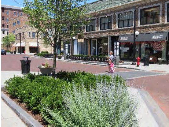
Typical raised planter at bump-out
